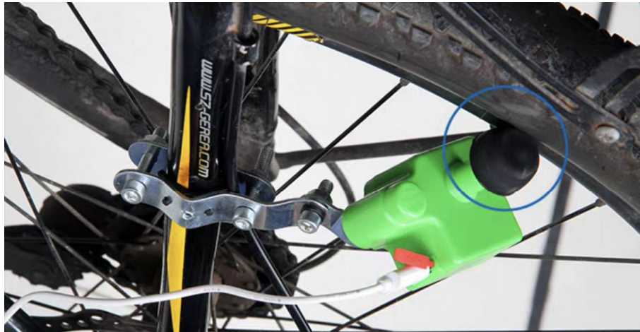
Figure 18: Installation of kinetic energy converter
